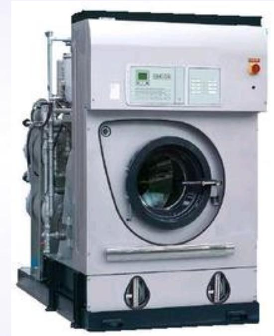
Because it is a flammable hydrocarbon all the machines will have closed circuit and distillation will be done with particular processes to avoid dangers of flammability. Hydrocarbon machine has a plan more or less similar to the one of perc.
